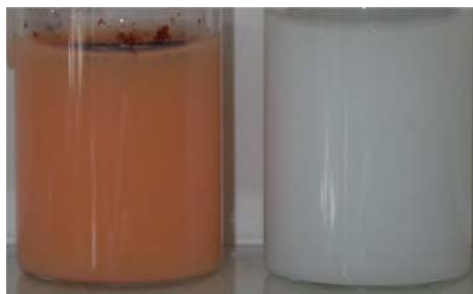
Photograph of the neat 100 nm latex (right) particles and the particles after dying by sorption with the hydrophobic pigment Sudan IV (left).
