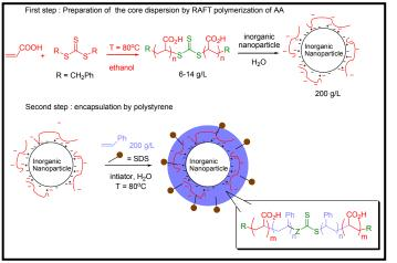
is then formed upon the addition of organic monomers via an emulsion polymerization process. The key feature of this encapsulation method is the use of a 'living' dispersant which is reactivated during the polymerization of the shell, thus leading to the formation of block copolymers. The shell is thus in effect covalently tethered to the dispersant, which is strongly adsorbed onto the inorganic nanoparticle surface.
