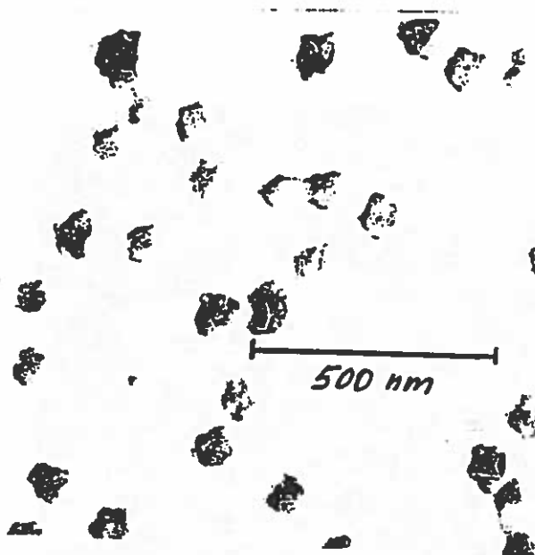
Fig.3 TEM of PMMA block copolymer particles (MMA 131)
