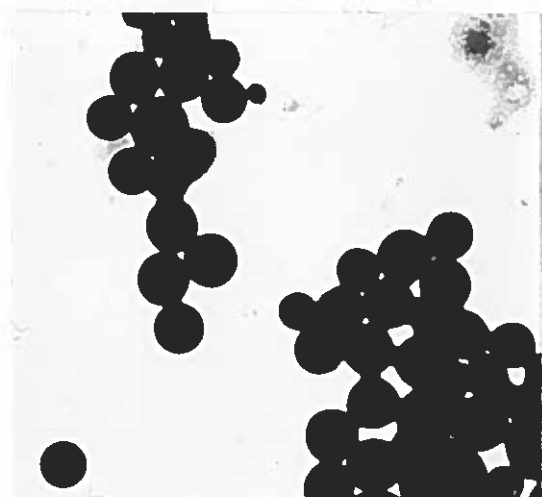
Fig. 1. Styrene monomer emulsion Styrene 300 g, H 2 O 1000 g Na cetylsulphate 2.15 g Cetyl alcohol = 6 g.
