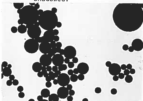
Fig. 4. Latex prepared by polymeri- zation of monomer emulsion shown in Fig. 1. Initiator K 2 S 2 O 8 .
